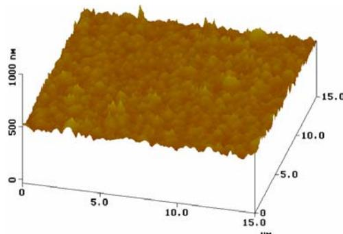
**Fig. 4(e).** Roughness of treated sample with aquaregia by 60 minutes.
