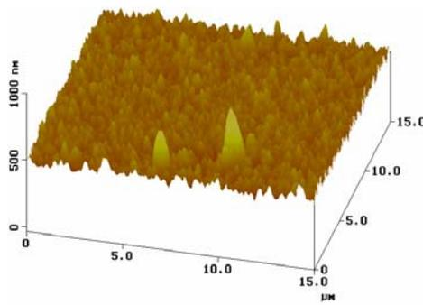
**Fig. 4(c).** Roughness of treated sample with oxygen plasma by 60 minutes.
