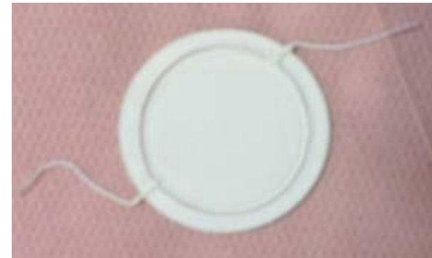
Ir/CGO catalytic layer (0.2 g)
